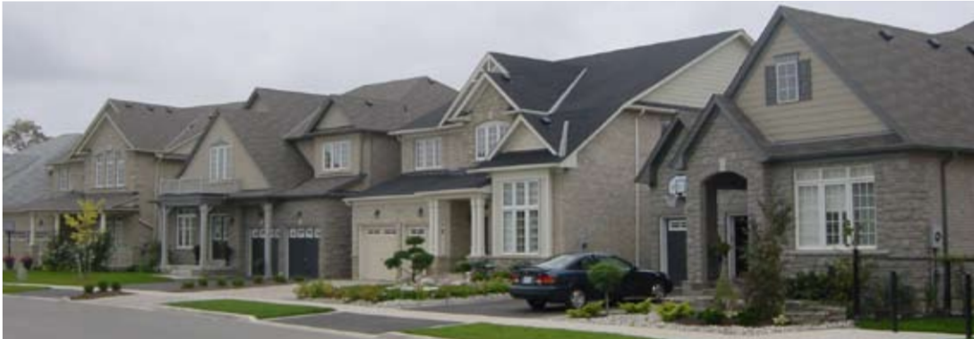
Figure 4.1c: The majority of attached garages in the streetscape shall be flush or recessed behind the porch or wall
