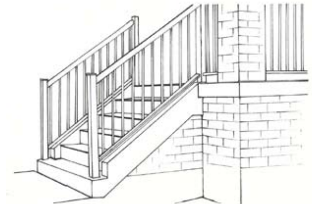
Figure 3.5c: Masonry veneer shall be applied to the side of main entry stairs, where more than 3 steps are required.
